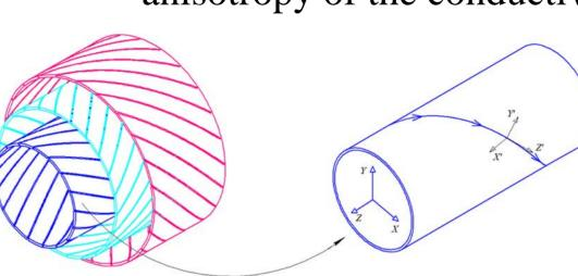
The conductivity of the anisotropic thin conductor is a tensor of order two, of which the off-diagonal elements are all zero.
