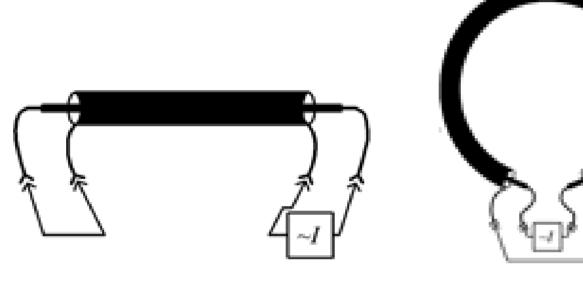
Two types of connections both sides of the cable.
