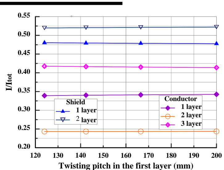
Calculated maximal currents in layers of the cable versus total current when the diameter of the third layer deviates from the optimal diameter by 0.1 mm that is just the thickness of one HTS tape.
