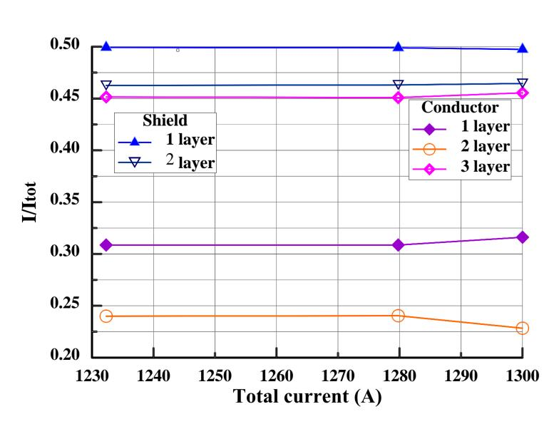
Measured current distribution between layers of conductors and shield of the HTS cable.
