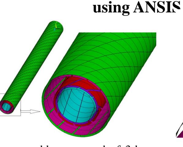
FEM of HTS power cable composed of 3-layer HTS conductor and 2-layer HTS shield.
