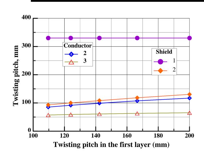
Twisting pitch in three-layer conductor and two layers shield for realizing homogeneous current distribution.
