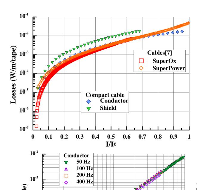
Comparison of AC losses per tape in compact cable and in another coaxial cables produced at VNIIKP.
