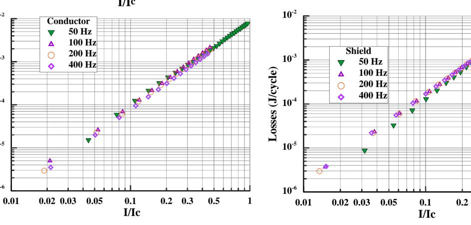
AC Losses at the conductor and shield at different frequencies.
