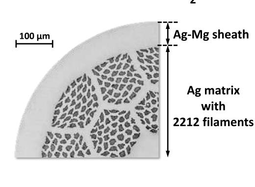
Increasing PO<sub>2</sub> during OP-PD decreases the grain size of the sheath
