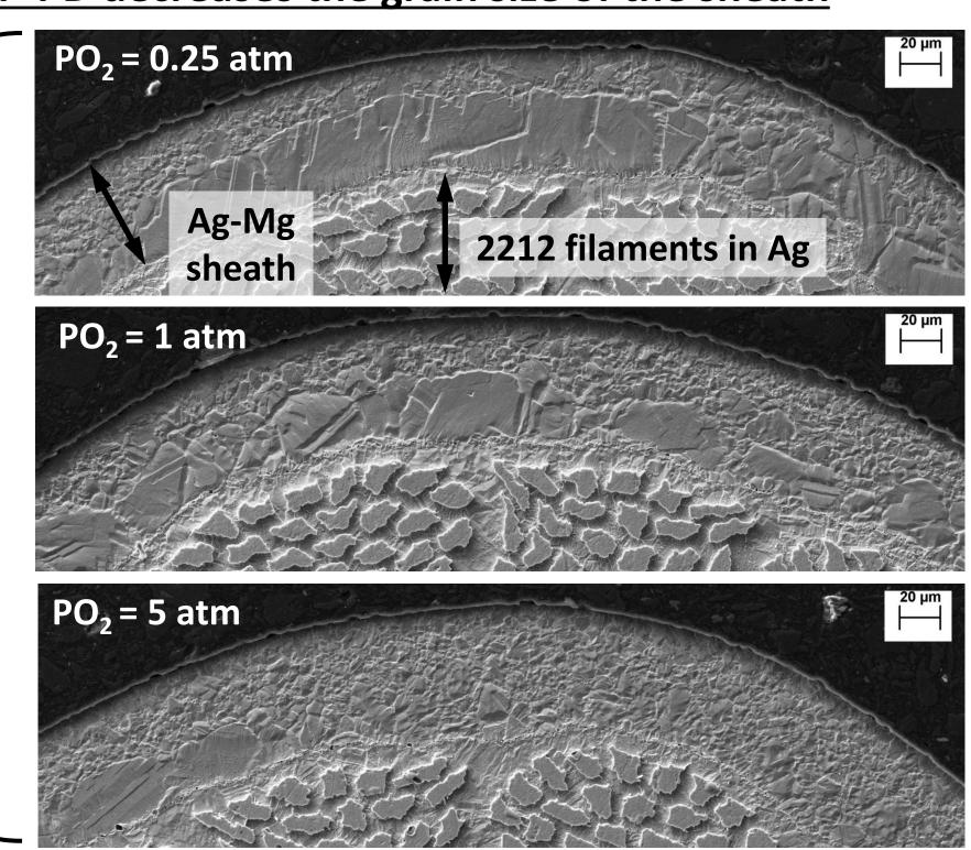
Scanning electron microscope images of chemically etched wire cross section
