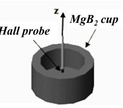
Superconducting cup: Outer radius: 10.5 mm Inner radius: 7.5 mm Ext. height: 10.5 mm Inner depth: 7.5 mm
