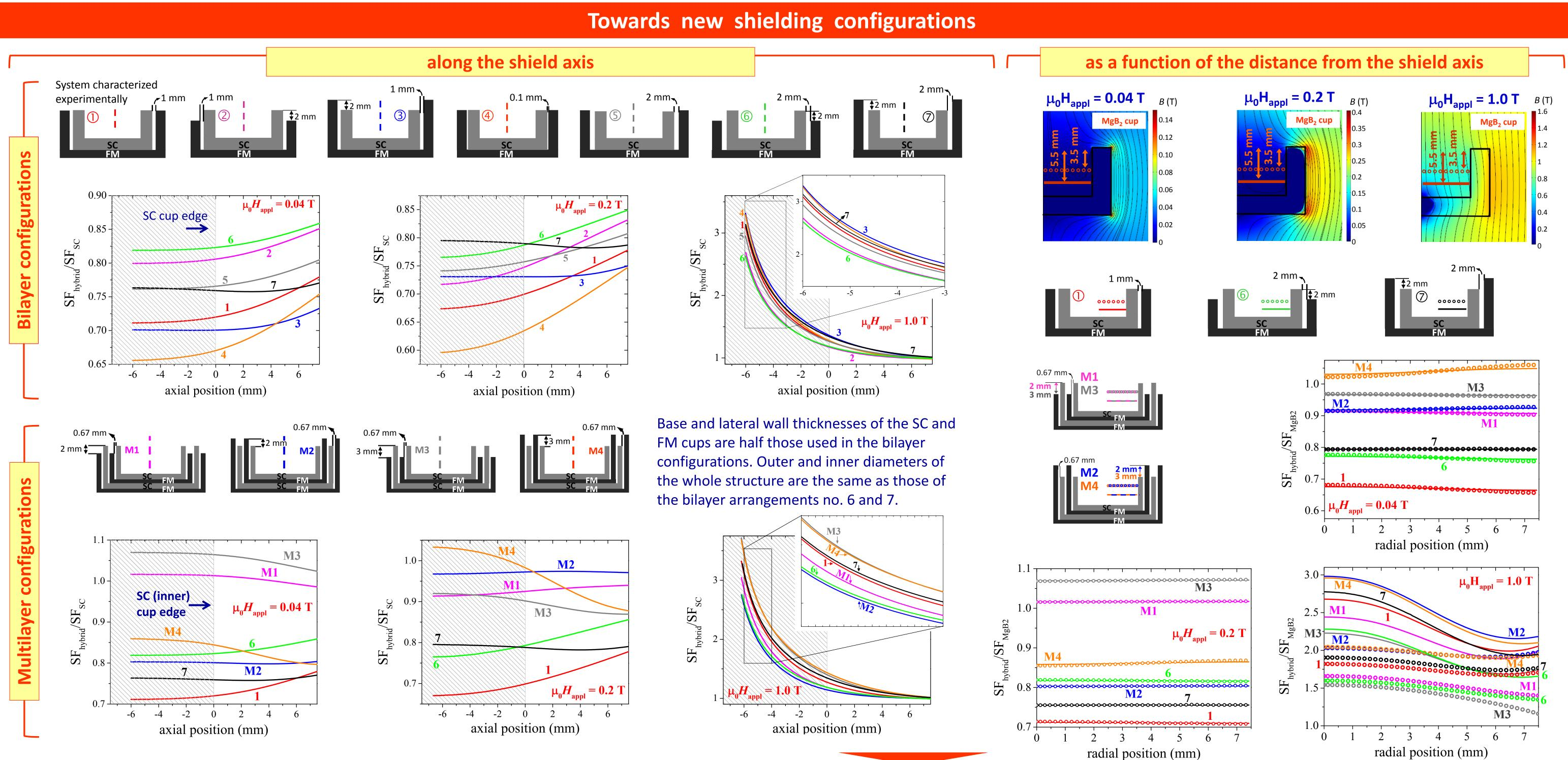
Multilayer configurations: higher shielding efficiency both at low and at high applied fields
