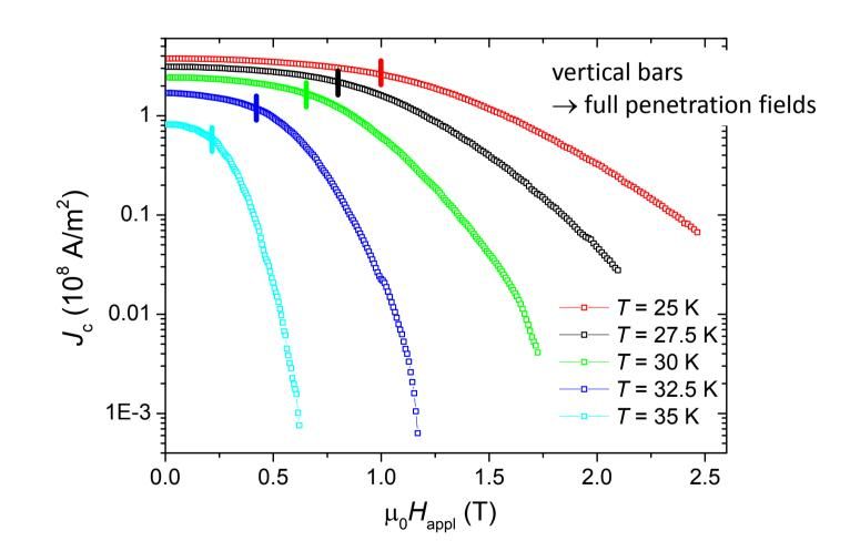
Critical current densities evaluated from the magnetic induction values, measured by the Hall probes along the tube axis in the axial field configuration, as [5]:
