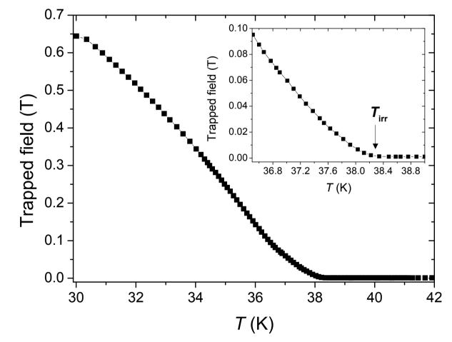
Temperature behavior of the field trapped in the center of the tube after the application of the external field  $\mu_0 H_{appl} = 1.2 \text{ T}$  (|| to the tube's axis) at T = 30 K.
