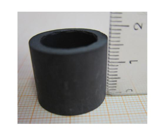
Outer radius:  $r_{out}$  = 10.0 mm Inner radius:  $r_{in} = 7.0 \text{ mm}$ Length: h = 17.5 mm
