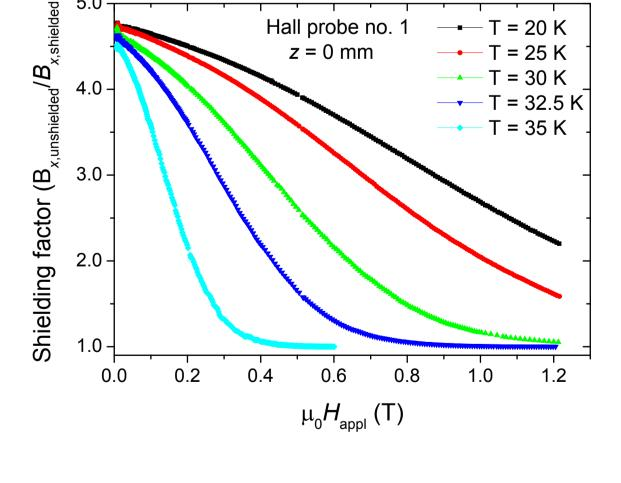
Shielding factor higher than (tube center):
