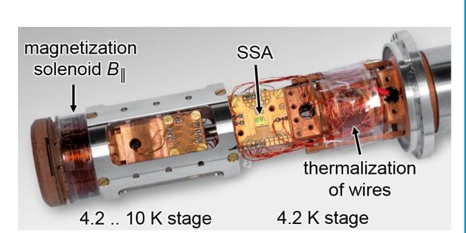
The SSA operates in magnetic fields of 100 µT in maximum and is therefore mounted approximately 6 cm away from the coil system.
