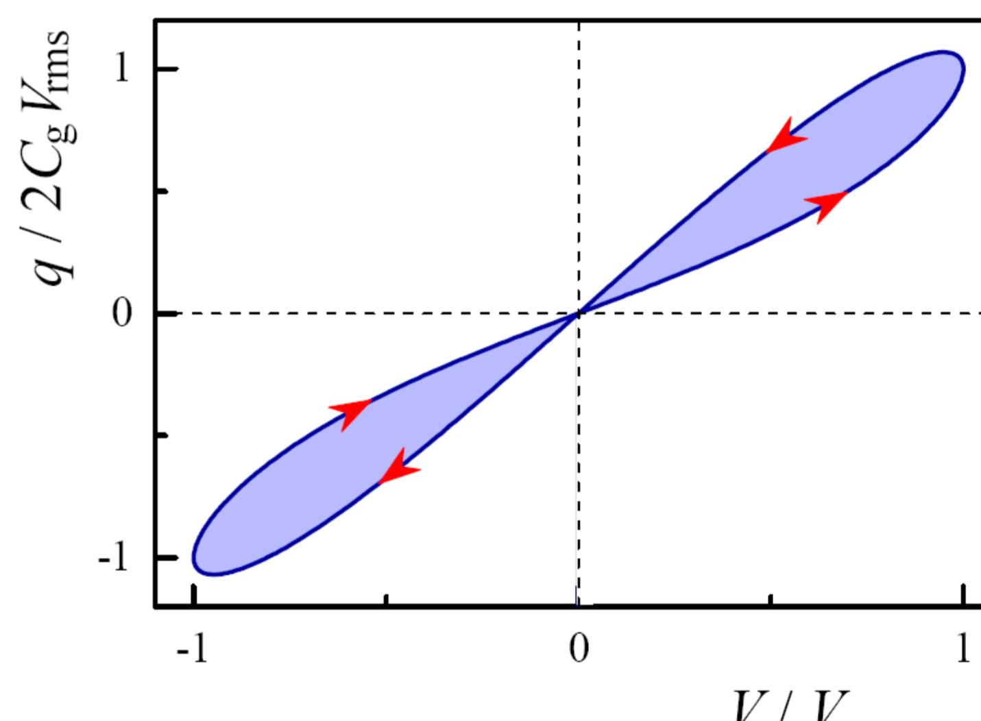
Pinched-hysteretic as a fingerprint of a memcapacitive behaviour
