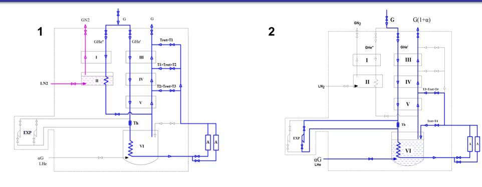
The cool-down scheme of the booster and collider. 1. the first stage, 2. the second stage
