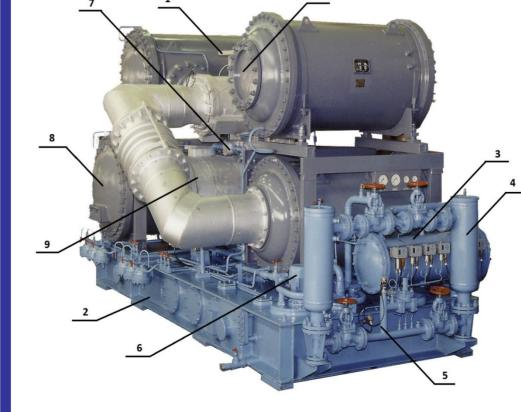
The nitrogen compressor "Aerocom2-179/18" specially designed by the JSC "NII Turbocompressor", Kazan, for the NICA complex:
