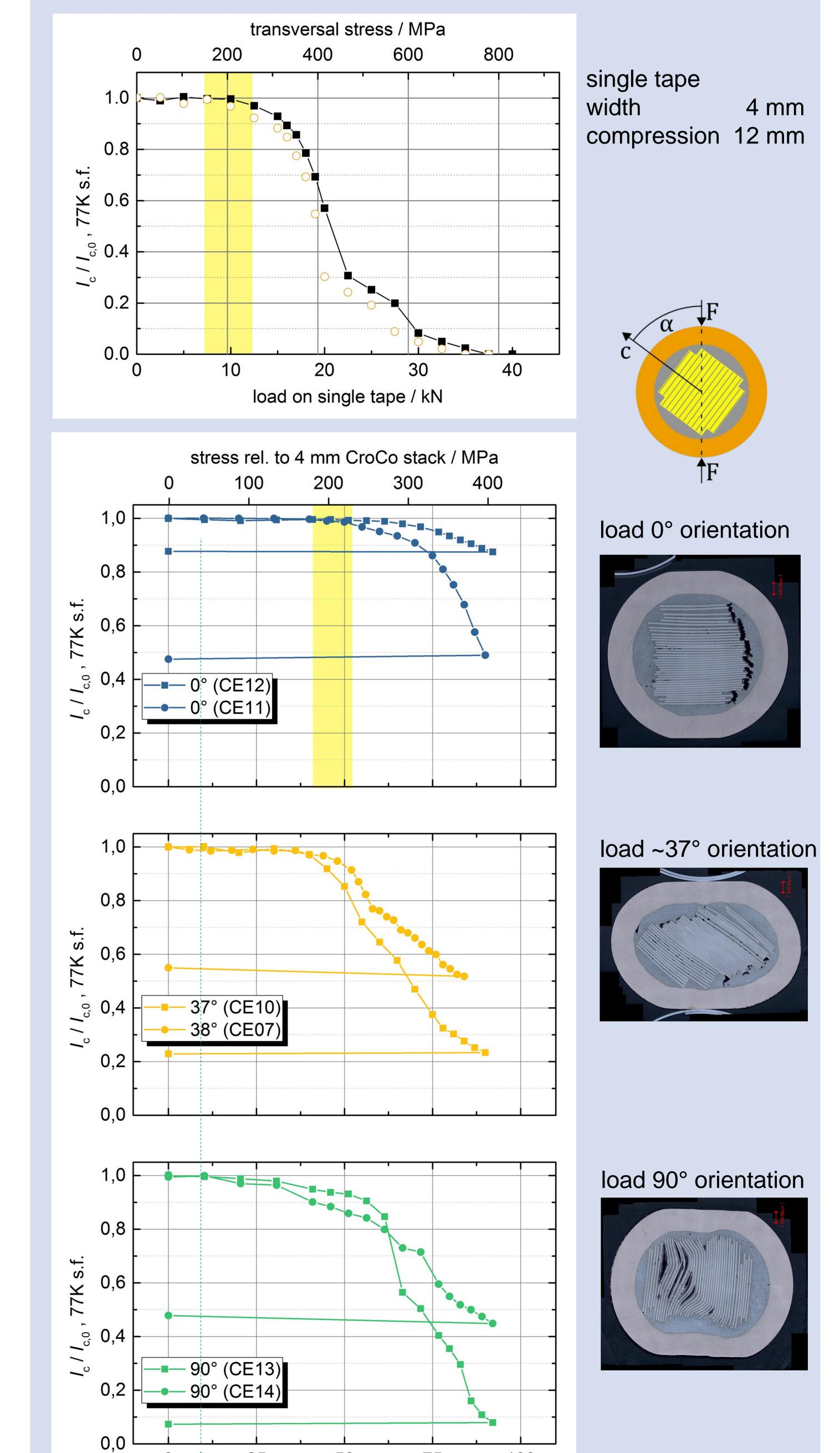
No degradation up to 10 kN ~  $F_{Lorentz}$  (80kA, 12T) / 6 CroCo on  $l_{2,comp}$
