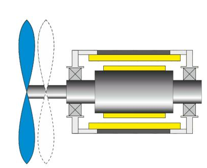
Application of racetrack HTS coils for field and armature windings
