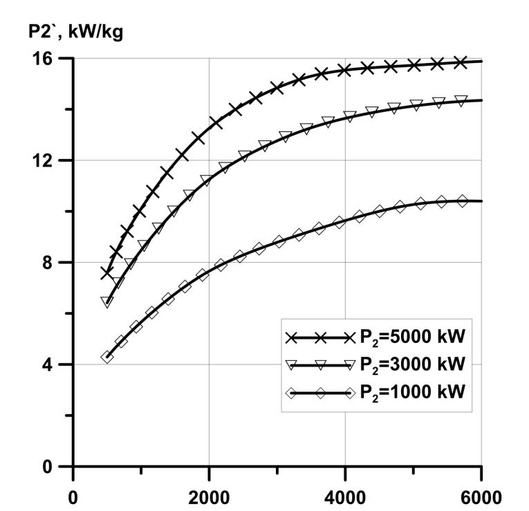
n, rpm Specific power vs rotational speed
