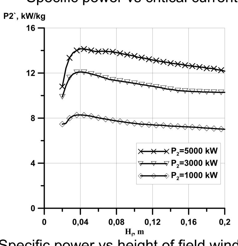
Specific power vs height of field winding
