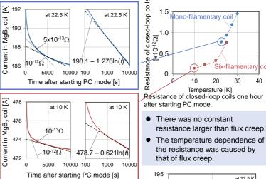
Current decay of closed-loop coils for three hours. ≤
