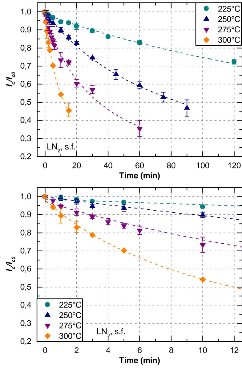
■ Degradation is strongly dependent on the temperature and time e.g. 10 % degradation after only 1 min at 300 °C. At 250°C 10 % degradation requires about 10 min
