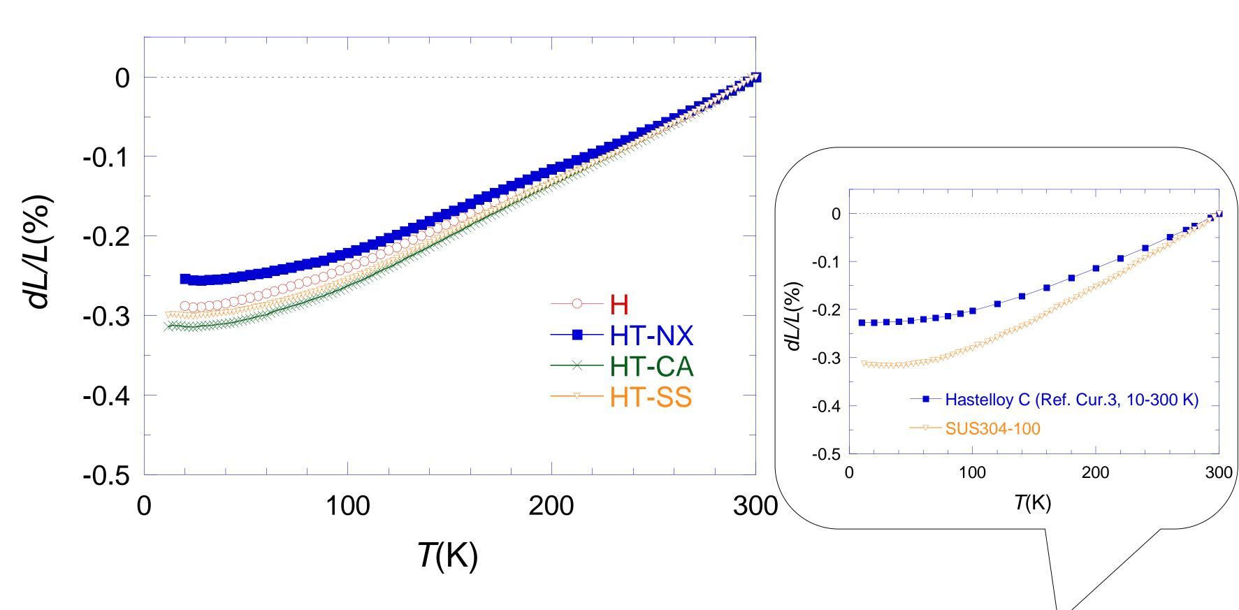
● The *dLL*(T) of the HT-NX tape is somewhat smaller than those of other tapes, which might originate from the small dLL values of a Ni-based alloy.
