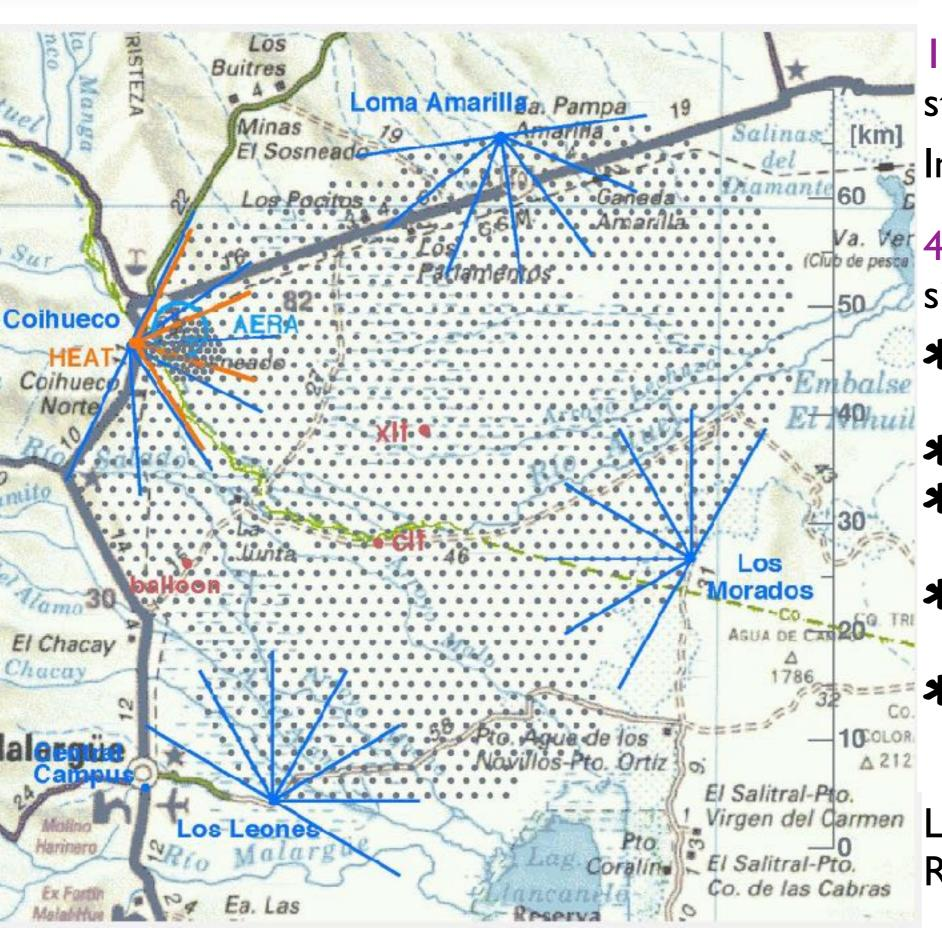
1660 surface detector stations, 1.5 km spacing Infill: 750m spacing
