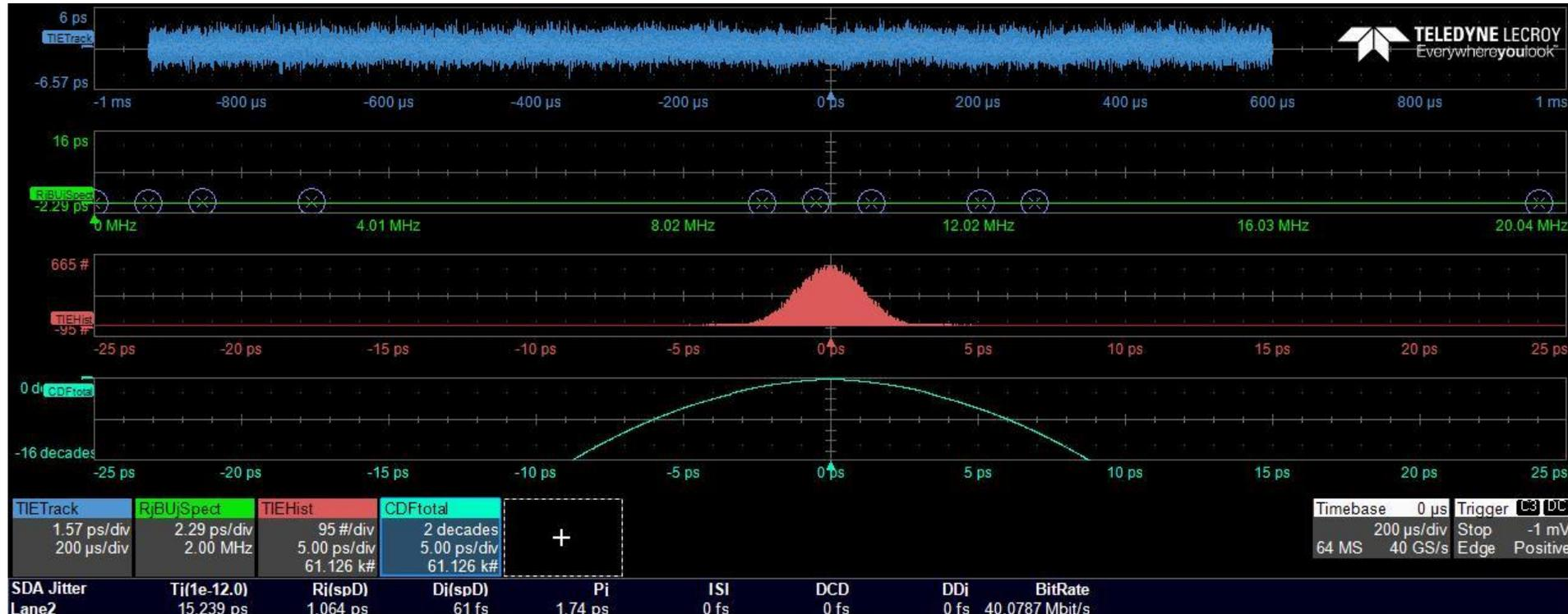
If no clock present on input of Si5345 => it generates free running clock 40.0785 MHz
