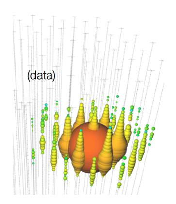
Isolated energy deposition (cascade) with no track
