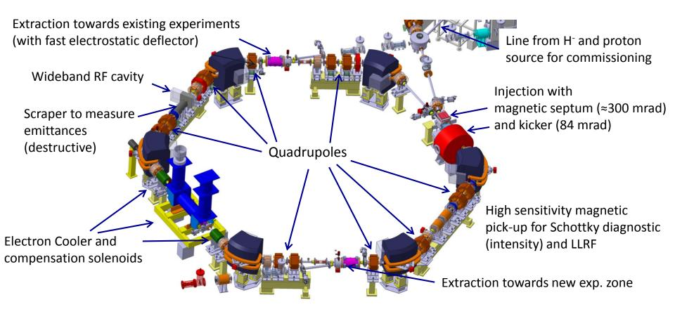
Deceleration of antiprotons from 5.3 MeV to 100 keV to improve efficiency of experiments
