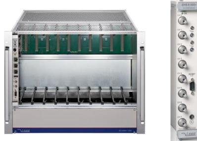
Up to 10 boards can be mounted in each chassis system, which can be mounted in universal 19" racks. A cooling system based on fans is provided and controlled by CPU.
