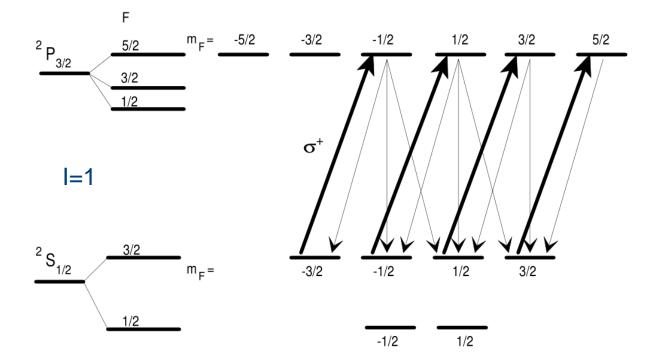
$\sigma^{\pm}$ : induces  $\Delta m_F = \pm 1$  transitions,  $\sigma^{\pm}$  was used for <sup>35</sup>Ar
