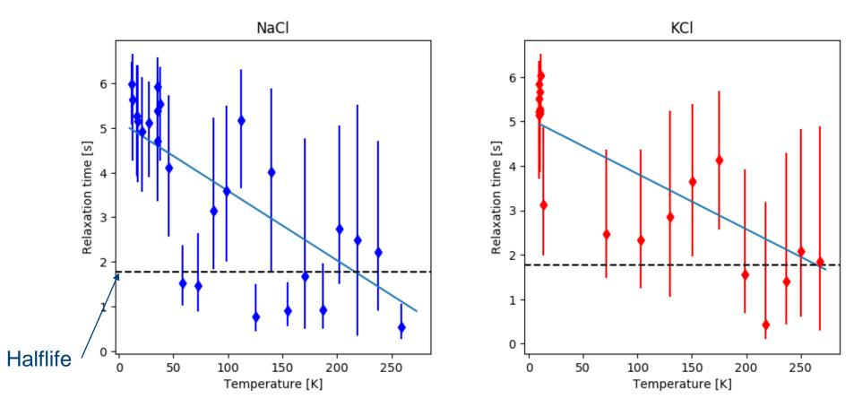
Upward trend/phase transition visible: possible freezing of Ar used to vent the beamline
