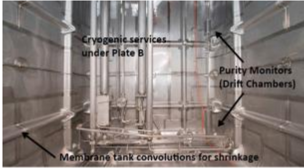
Non vacuum insulated membrane cryostat
