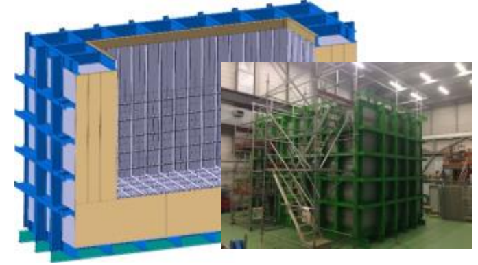
30 m 3 Dual Phase prototype at CERN (operational at CERN)
