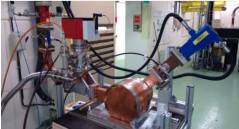
Figure 8: Setup of the high power test of the RJ in CTF2 at CERN.
