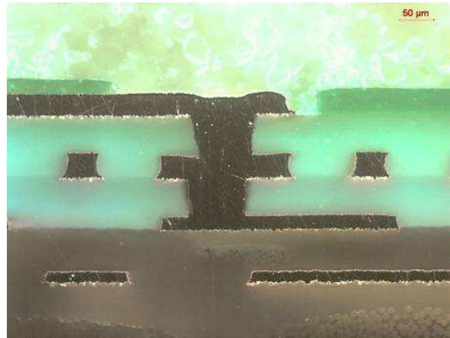
Stacked laser microvias copper filled
