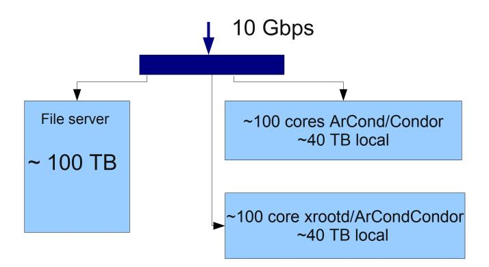
PC farm nodes are based on Dell PowerEdge R710 (2 processors, Xeon 5520 (8 cores) + 2.5 GB per core + 4TB local data disks)
