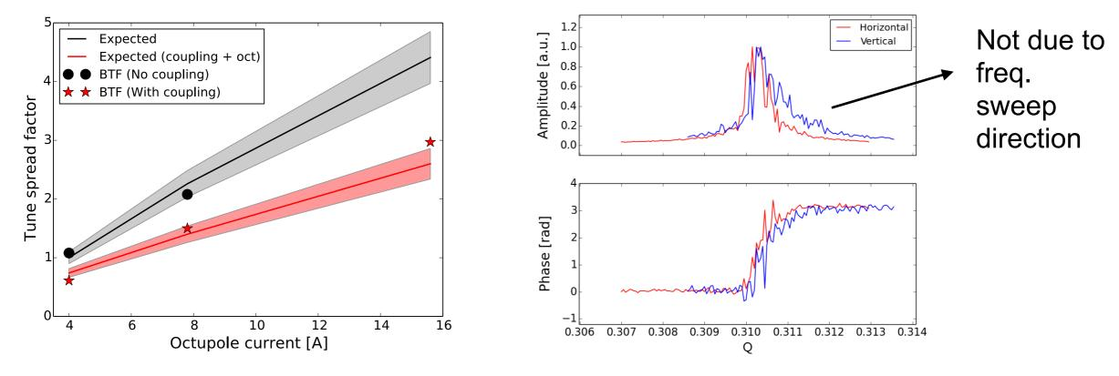
We want to characterize the Landau damping at flat top energy for different octupoles currents, tunes and linear coupling values and beam-beam effects
