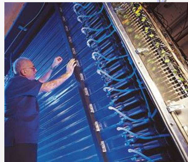
Michigan University: 'neutron wall'. The flat-sided glass tubes contain liquid scintillator.
