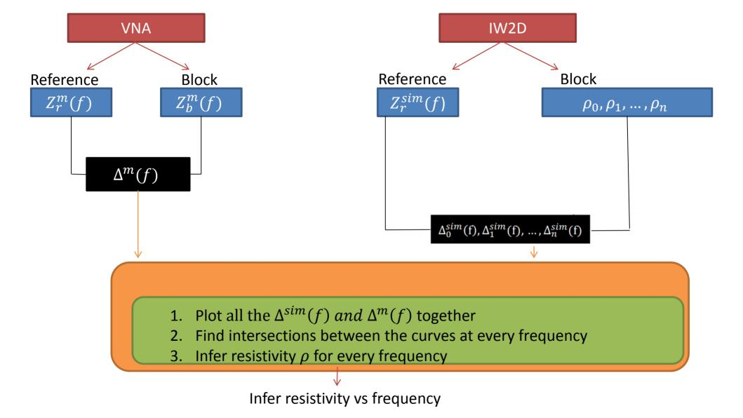
Resistivity measurements on collimator blocks routinely performed in the lab.
