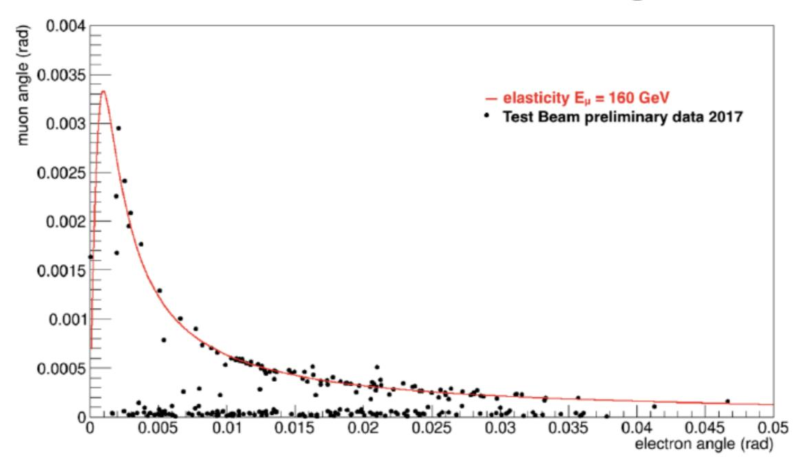
160 GeV muon beam, 8 mm C target Golden selection: single track in and two tracks out
