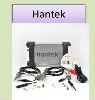
+ 4 ch Oscilloscope- No GPS, no trigger logic
