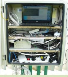
Detectors data acquisition with the Quarknet card based on the Time over Threshold technique
