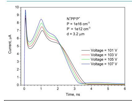
The current pulse shape and duration is quite different in P- and N-type diodes mainly due to the difference of the electric field in the region with low impurity density  $(N^-,P^-)$  and due to the difference of the ionization coefficient of electrons and holes ( $\alpha_e \cong 10\alpha_h$ ). But charge collection is almost the same in the absence of traps.
