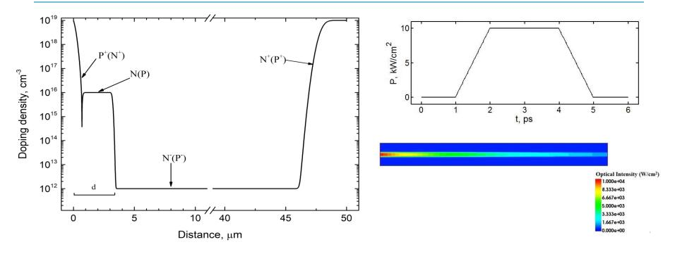
Drift-diffusion model according to Synopsys TCAD Sentaurus. Shockley– Read–Hall (SRH), Auger, recombination through two deep levels, and charge generation due to impact ionization (the van Overstraeten and de Man model) was taken into account.
