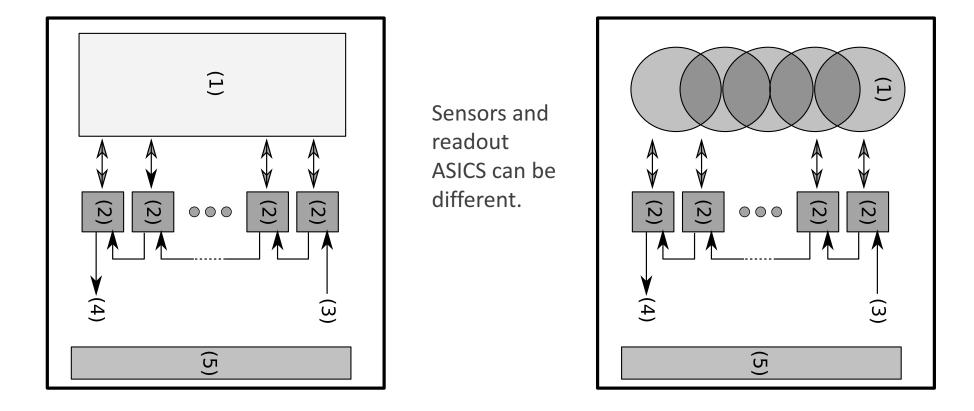
The input/output plus voltages go through connector (5)
