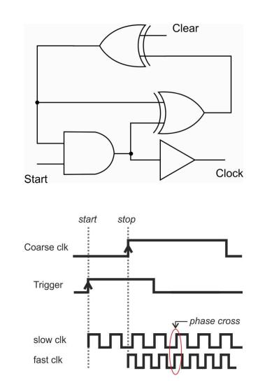
A Vernier TDC embedded in the FPGA
