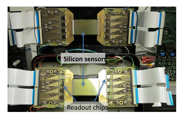
Yet another **stack of silicon pad detectors** for a PET probe
