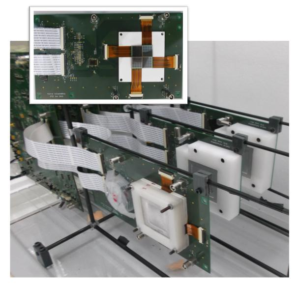
A **stack of Scintillarors+SiPM** for a Compton Telescope to monitor hadron therapy.
