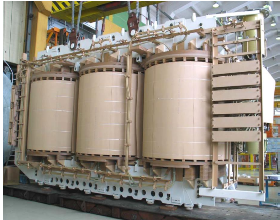
Conventional 400 MVA Transformer
