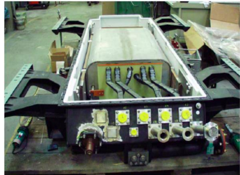
Transformer installed in frame
