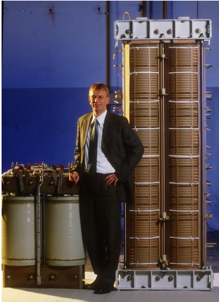
HTS-Train transformer left Normal train transformer right
