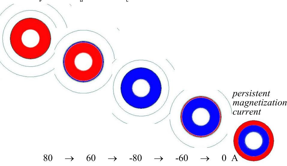
AC transport in hard superconductor is not dissipation-less (AC loss)
