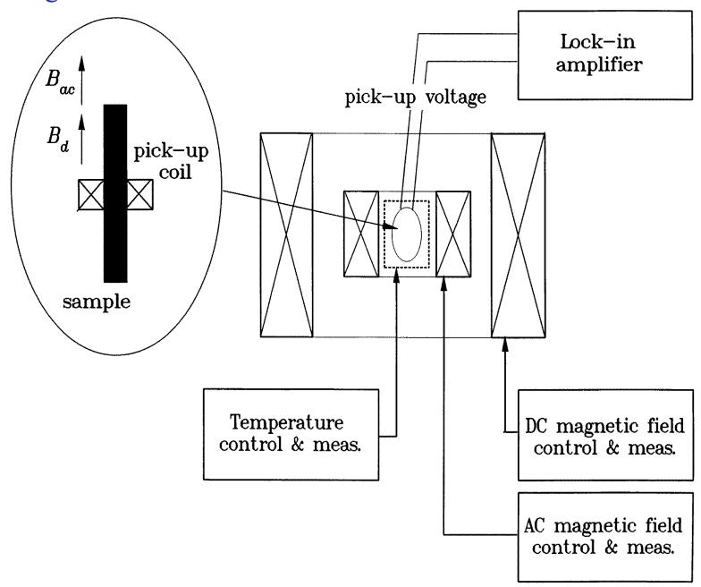
pick-up coil wrapped around the sample induced voltage  $u_m(t)$  in one turn:
