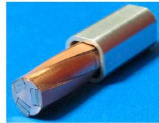
20 YBCO tapes in each helical groove in a copper diameter 9.5 mm.
