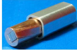
40 YBCO tapes in a copper diameter 9.5 mm.
