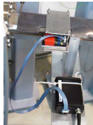
Figure 1: Installed PIN Diode Beam Loss Monitor with its power supply.
