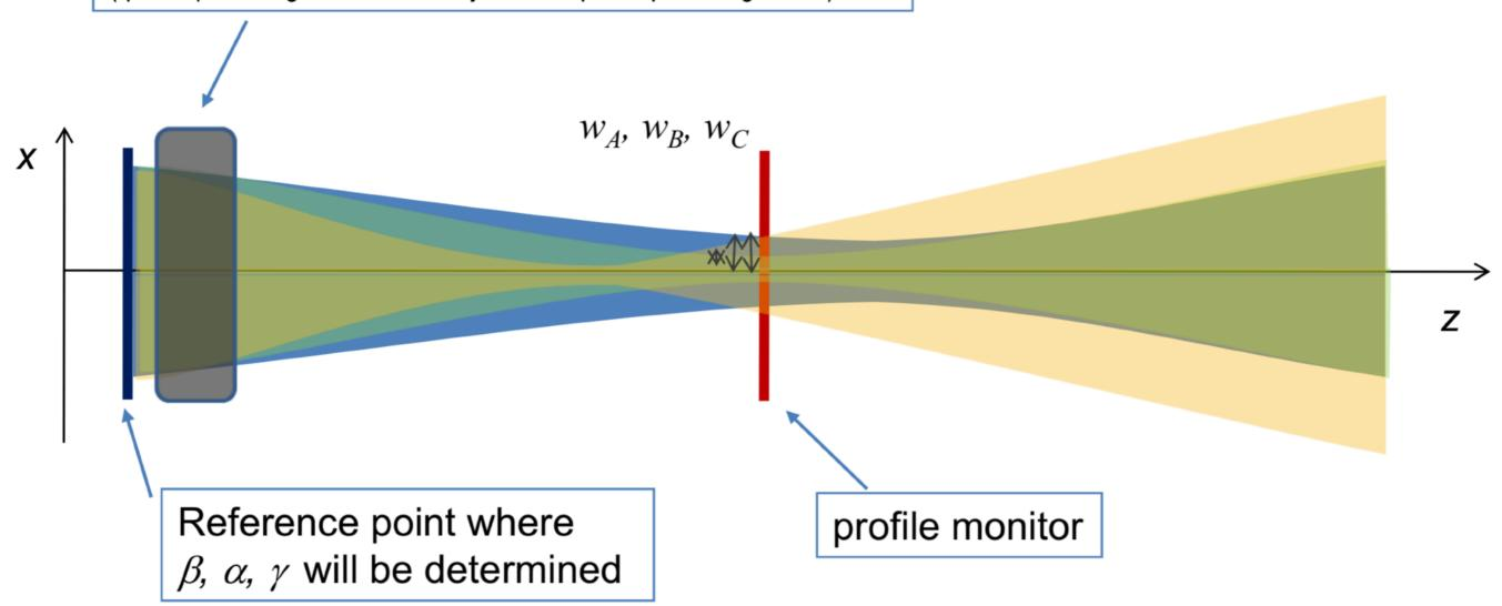
$$\begin{pmatrix} c & s \\ c' & s' \end{pmatrix} = \begin{pmatrix} 1 & L \\ 0 & 1 \end{pmatrix} \cdot \begin{pmatrix} m_{11}(I_{mag}) & m_{12}(I_{mag}) \\ m_{21}(I_{mag}) & m_{22}(I_{mag}) \end{pmatrix}$$
