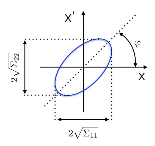
$$\Sigma = \begin{bmatrix} \Sigma_{11} & \Sigma_{12} \\ \Sigma_{12} & \Sigma_{22} \end{bmatrix} = \begin{bmatrix} \langle x^2 \rangle & \langle xx' \rangle \\ \langle xx' \rangle & \langle x'^2 \rangle \end{bmatrix}$$
