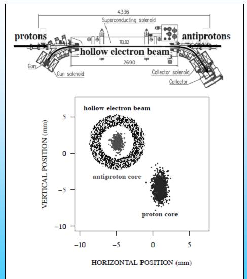
Figure 3: Schematic diagram of the beam layout in the Tevatron hollow electron beam collimator.
