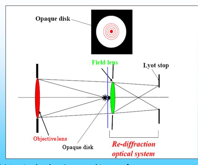
The first lens (objective lens) makes a real image of the object (beam image) on to a blocking opaque disk
