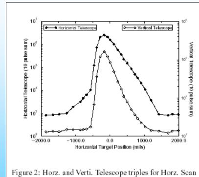
Solid angle remains the same through scan Narrow acceptance, reduces noise.
