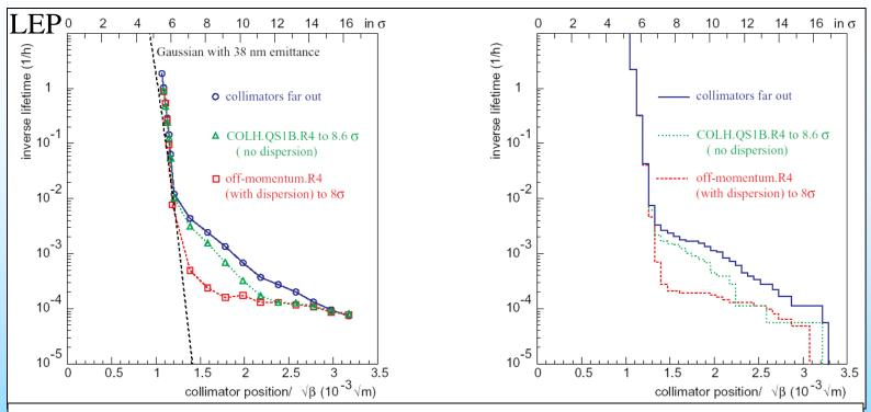
Measurement (left) and simulation (right) of the horizontal beam tails for a beam energy of 80.5 GeV and for different collimator settings at LEP. The simulation is the result of tracking particles after Compton scattering on thermal photons (black body radiation of vacuum chamber).
