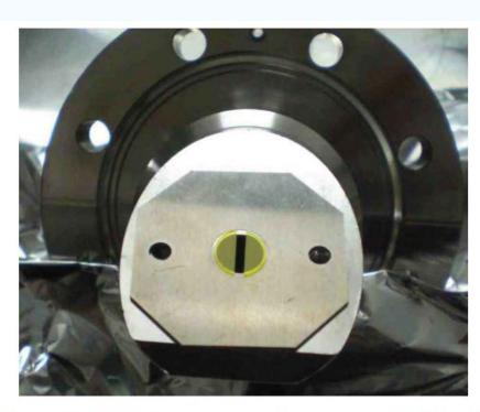
Figure 2: YAG:Ce screen on the actuator holder: The beam core goes through a slit at the center of the screen without any interaction for the scintillator.
