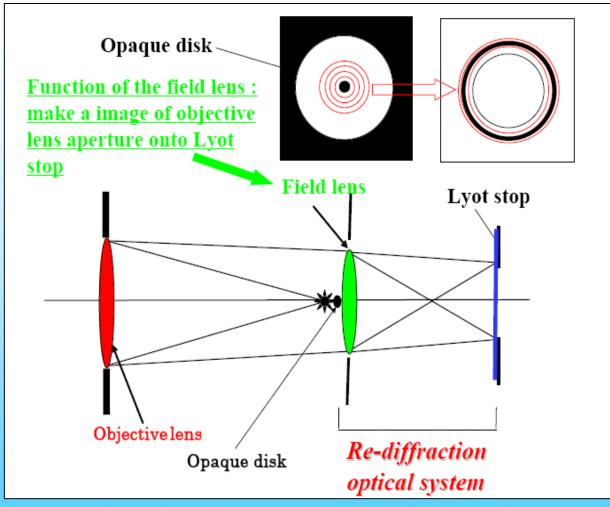
A second lens (field lens) is set just after the blocking disk. The focusing length of the field lens is chosen to make a real image of the objective lens aperture onto a mask (Lyot Stop).
