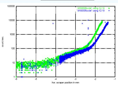
Beam loss rates versus scraper position, black: first measurement, grey: second measurement. During the second measurement the orbit moved about 0.30 mm in 4721 s.
