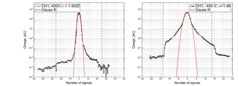
Fig. 14. Measured beam core and beam halo distributions using the DSv, with cuts by apertures in the horizontal (left, BX10BY0.5 optics) and vertical (right, BX10BY1 optics) planes. The positions of the cuts obtained in the simulation from the tightest apertures are indicated by dashed lines, for a perfectly aligned and optically matched beam.
