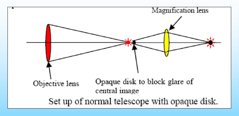
When using OTR or SR (narrow cone) the diffraction fringes makes tail surrounding from the central beam image. Intensity of diffraction tail is in the range of  $10^{-2}$  - $10^{-3}$  of the peak intensity. The diffraction tail disturb an observation of week object surrounding from bright central beam
