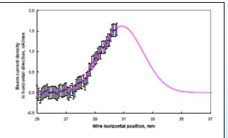
Scan of the electron beam at the Injector of Yerevan Synchrotron with an average current of about 10 nA (after collimation) and an electron energy of 50 MeV
