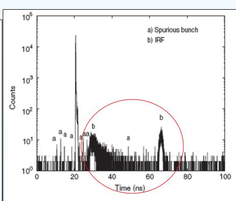
Fig. 5. SRS single bunch mode pattern at 600 MeV. Due to a small current (4 mA) the count rate is only 3000 and the background is 100 counts/s. Spurious bunches (a) can be seen in the adjacent buckets of the main bunch, and the after-pulses of the MCP-PMT (b) as observed in the IRF.
