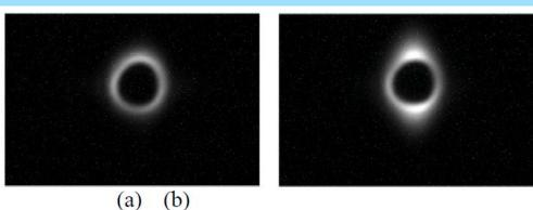
Figure 8: Result of two images taken by coronagraph for vertical, (a) original beam profile (no excitation of blew up) and (b) blow up to 10 µm.
