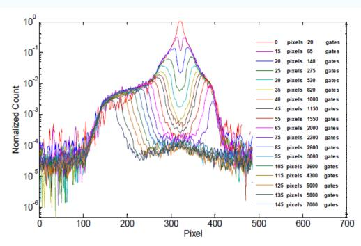
Figure 6: Measured beam profile with different mask sizes. Background subtraction and signal averaging was
