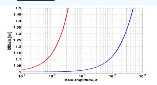
Figure 3: Dependence of the RMS size (blue line) and of the kurtosis (red line) on the halo amplitude for the profile
