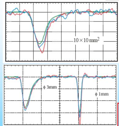
APD: The average over many events is shown (smooth curve) as well as two single-photon events to show an indication of the noise level Scale: 50 mV (upper) 100 mV (lower) and **5 ns /div.**
