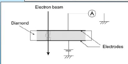
Figure 2: Principle of the diamond-based detector.
