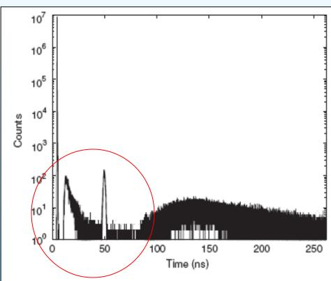
Fig. 4. Full scale of the IRF recorded with the 35 ps diode, with approximatively 1 count/s noise.
