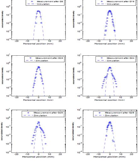
Simulation and (wire-Scanner) measurements at the beam transport line at the end of the IHEP RFQ.
