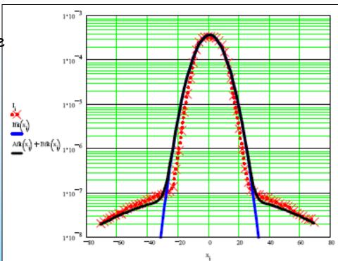
A normal function shown in solid blue has been fit to the data (red x's). A sum of two normal functions is shown in solid black. The x-axis is scaled as scanner position in mm's and the y-axis is log-amp input current in Amps.
