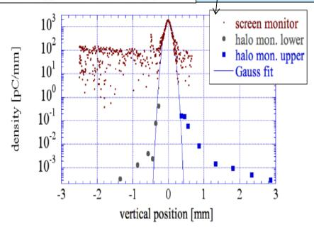
Figure 17: Vertical beam profile measurement by using the halo monitor and the screen monitor.
