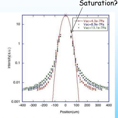
Figure 8: Distribution of the beam halo for the different vacuum condition in the case of the beam intensity  $0.45 \times 10^{10}$  electrons
