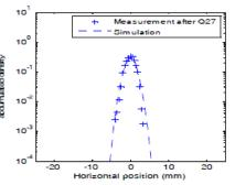
From the Figure 2 we can see in the most locations the simulations can properly reproduce the beam profiles, and there are a little halo particles in two locations. That means the beam in the phase space is not elliptic symmetry.
