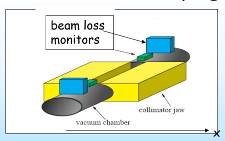
In a synchrotron one jaw will scrape both sides of the beam distribution ( $\beta$ -oscillation) => meas. symmetric halo Such a tail scan yields information about particles which oscillate with an amplitude larger than the position of the collimator = Halo Scraping
