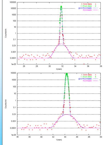
Figure 4: Beam Profile combining the  $25\mu m$  and 1mm Fe wire data. The top(bottom) plot shows the X(Y) data and results of the fit to the data. The red points represent the 1mm wire data, the green points the  $25\mu m$  wire data, the blue curve is the overall fit to the data and the red curve is the halo portion of the fit. The ordinate is plotted with a log-scale and the count rate is normalized to the beam current.
