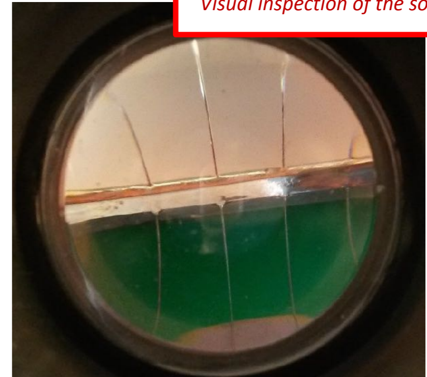
Test of grid brazing
