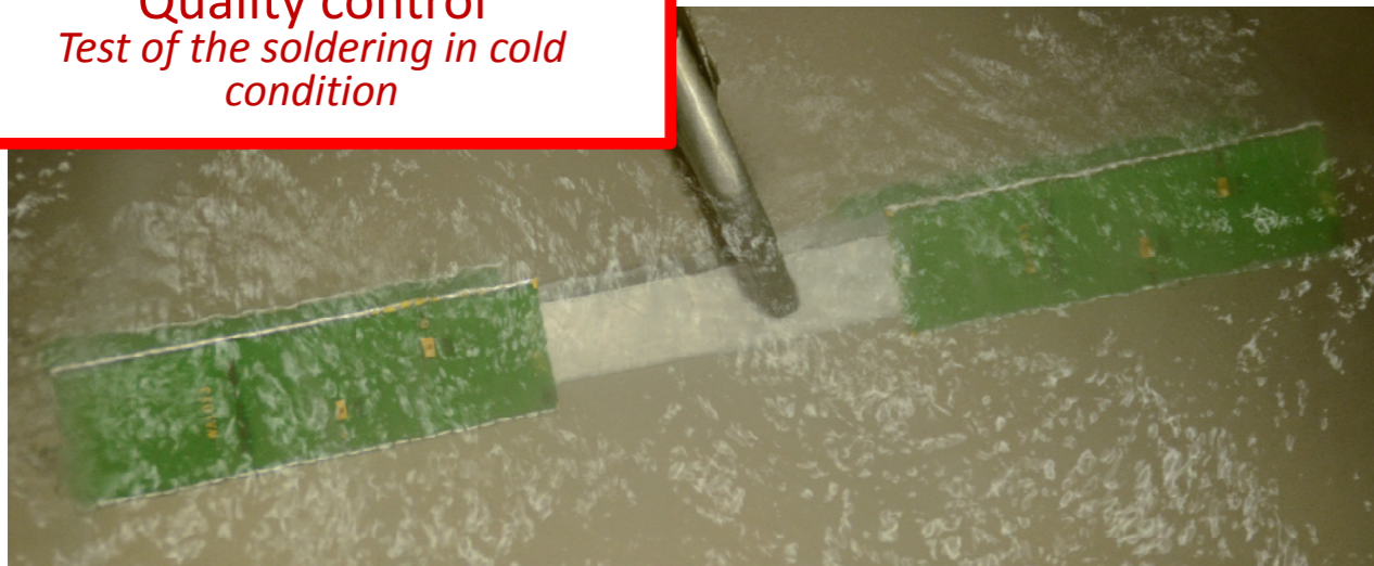
Grid prototype in liquid nitrogen, for cold test of the brazing
