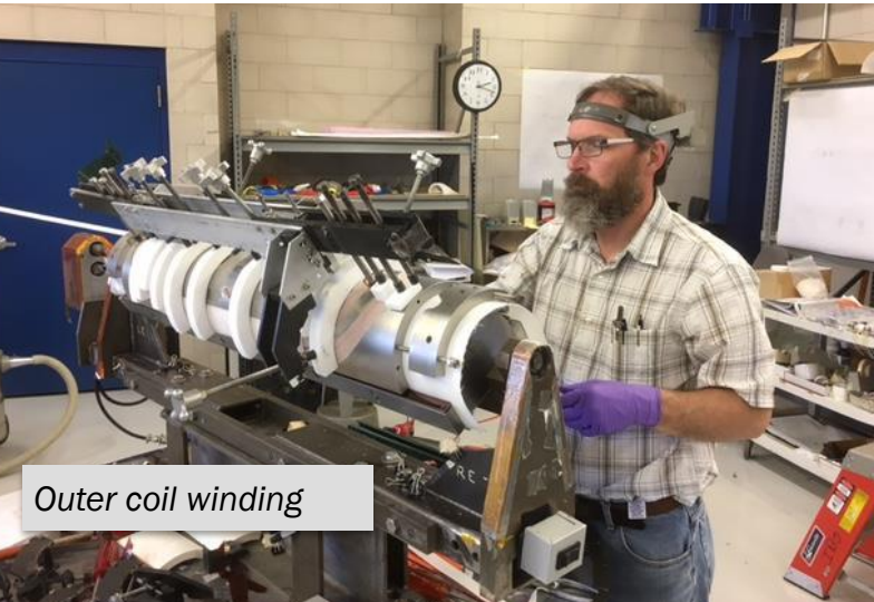
Novel coil layout addressing midplane stresses and field quality
