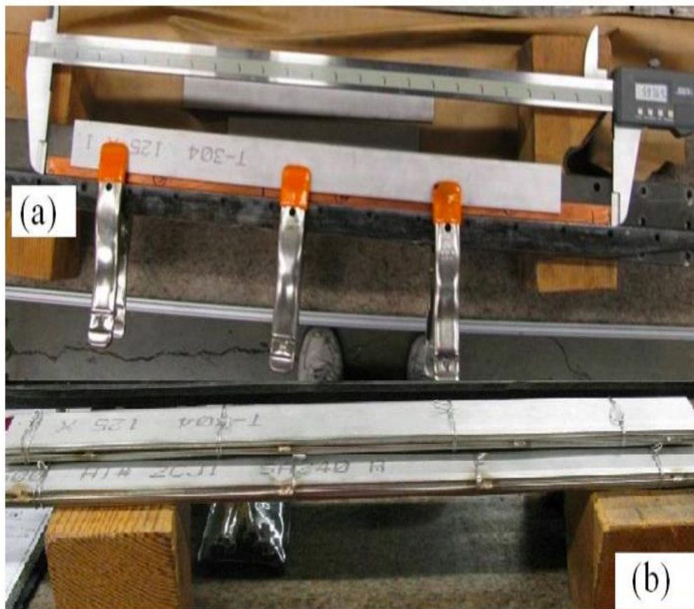
Figure 7: a) Measuring cable length, b) in the unconfined case, the cables are placed between siderails, top & bottom plates are tied together
