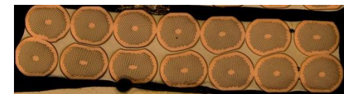
1 mm, 192 tubes PIT from Bruker EAS
