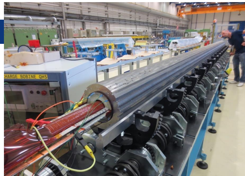
5.5 m long collared coils
