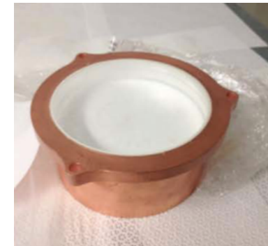
2 kg test crystal @U. Chicago. Amcrys-H, Ukraine
