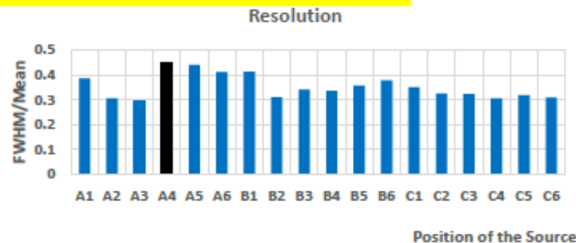
Uniformity scan performed after A4 was illuminated for 67 hours
