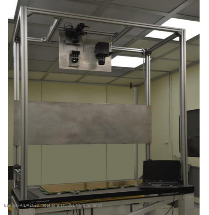
d setup for large flatness Engineered foils MPGD monitoring
