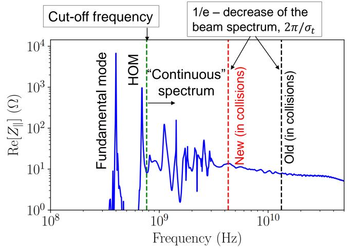
HOM parameters:  $f_r \approx 694$  MHz,  $R/Q \approx 10 \Omega$  (CST EMS simulations)  $\rightarrow$  Only one mode below cut-off frequency can affect power losses
