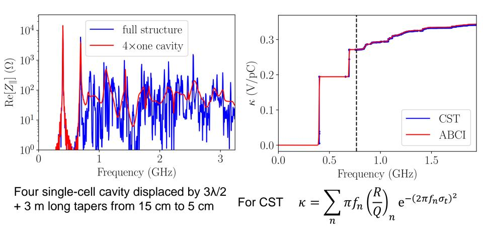
There are still a few modes below cut-off frequency of the cavity with high R/Q. Higher frequency HOMs have small R/Q values
