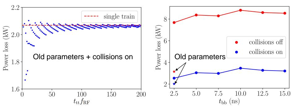
Power loss is moderate for the present cavity design for bunches in collisions There is a weak dependence on train spacing and bunch spacing
