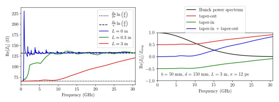
For  $c\sigma_t \ll b \ll d$ , impedance of step transition at high frequencies
