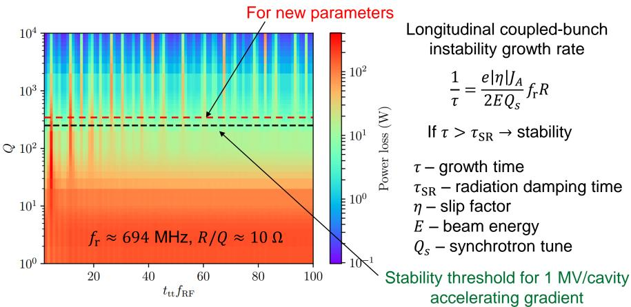
Power losses of few 100 W are for small Q + "resonant" cases with high Q  $\rightarrow$  Damping of the mode for longitudinal stability should moderate  $\rightarrow$  Resonant cases should be identified 10
