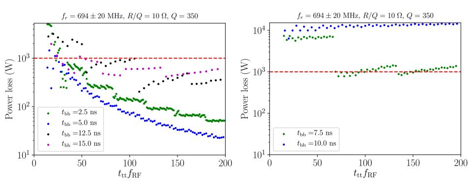
$\rightarrow$  More values of train spacing should be avoided in operation  $\rightarrow$  Strong power losses for 7.5 ns and 10 ns bunch spacings
