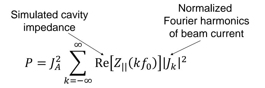
$J_A$  – average beam current  $f_0$  – revolution frequency k – revolution harmonic number
