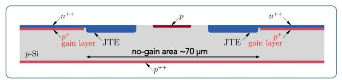
present limit of no-gain area in the UFSD design 70-100 µm
