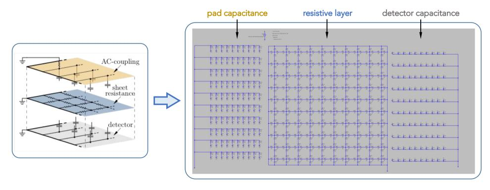
How large should the AC pad be so that the signal is similar to the input current, still having a large coupling capacitance?
