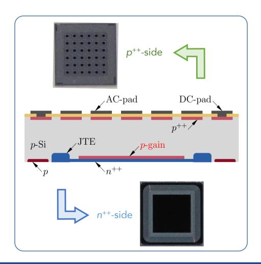
Besides *n*-segmentation, the first UFSD production at FBK (300  $\mu$ m) also accounted for *p***-side segmentation**.
