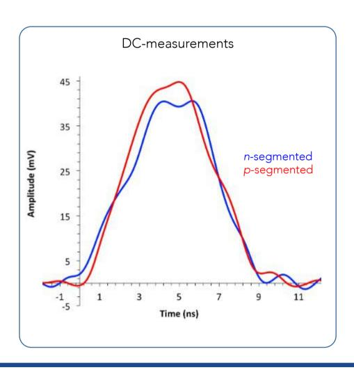
Besides *n*-segmentation, the first UFSD production at FBK (300  $\mu$ m) also accounted for *p*-side segmentation.
