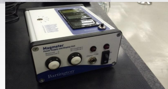
Bartington fluxgate with battery-operated 3-axis display unit (various models, lowest range is 70 nm to 70 \mu m, up to few kHz analog out)
