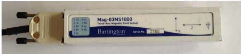
Bartington 3D fluxgate Bartington Mag-03MS1000 Range: 0 to 10 G, resolution 0.01 G
