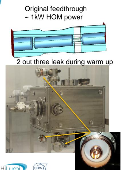
Replacement feedthrough Installed in mid-July
