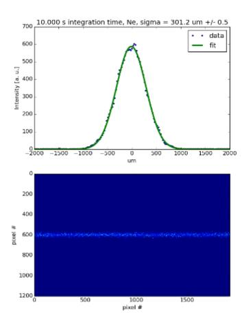
10 sec integration time. Magnification 0.25 Relative error on sigma 1% to be confirmed
