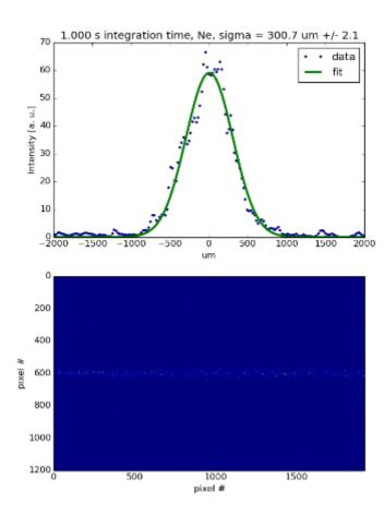
1 sec integration time. Magnification 0.25 Relative error on sigma 3% to be confirmed
