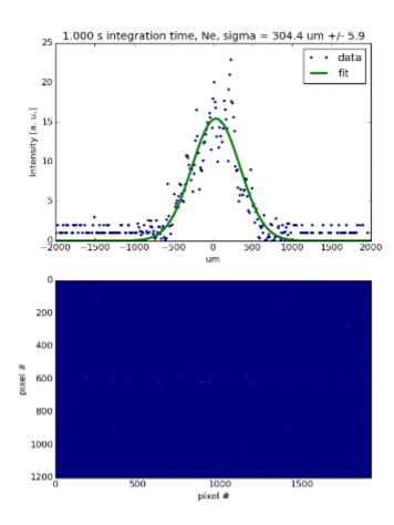
1 sec integration time, approx. 500 photons Relative error on sigma 3% to be confirmed
