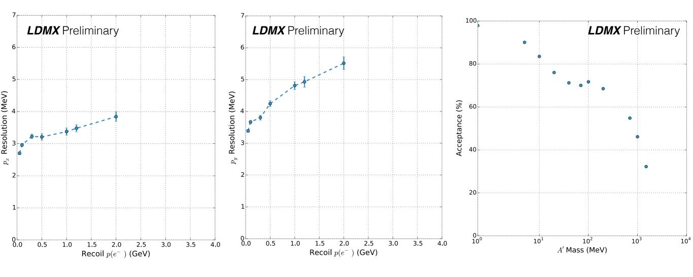
resolution limited by 4 MeV from multiple scattering in (full) target  good acceptance over wide mass range
