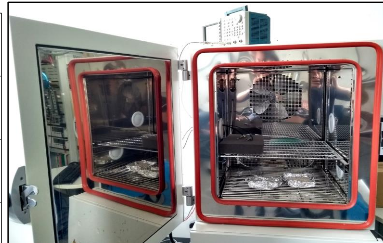
Test of LNA and other antenna components in special fridge
