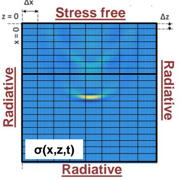
Irradiation by laser pulses, below ablation threshold Nd:YAG, 7 ns,  $\sim 0.1 \text{ J}$
